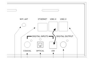
To ensure optimal Wireless performances, screw the provided wireless Antenna.
